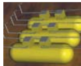
The presence of three abandoned underground storage tanks were detected by Landsweep™ on a brownfield site
