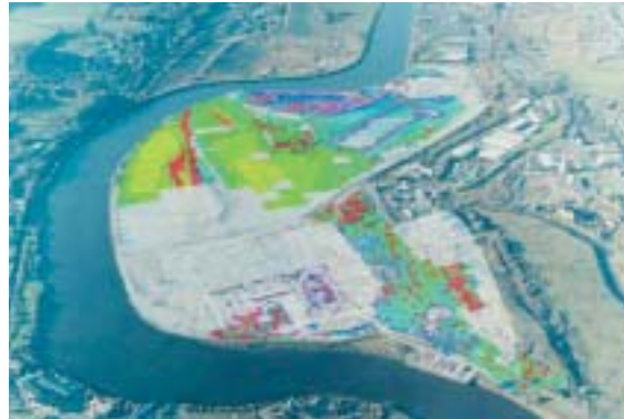
Landsweep™ detected and mapped many previously unknown features on this brownfield site in Northeast England
